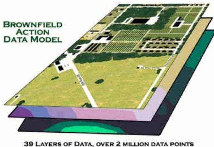
**FIGURE 2.** Data can be obtained for surface and bedrock topography, water table, water chemistry, soil characteristics, and vegetation as well as data from tools like soil gas, seismic reflection and refraction, metal detection and magnetometry, ground penetrating radar, and drilling.
