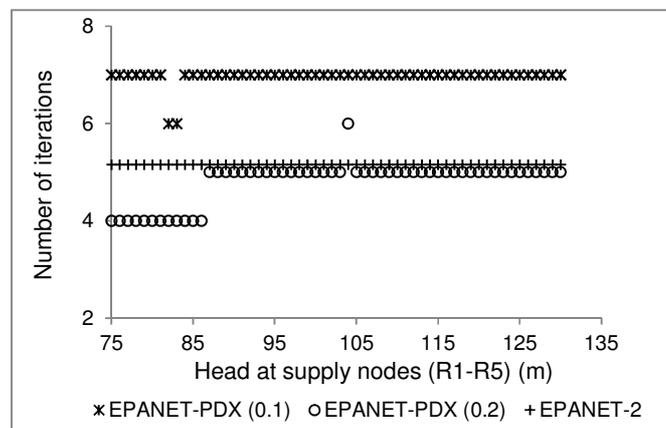
Figure 3. Number of iterations required as a function of the available pressure in the network
