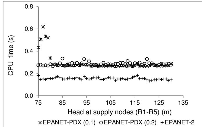
Figure 4. Comparison of CPU times for EPANET 2 and EPANET-PDX
