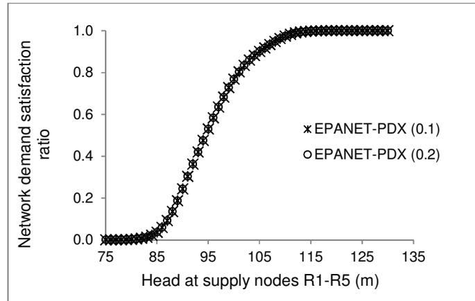
Figure 2. Influence of variations in supply node heads on the flow delivered
