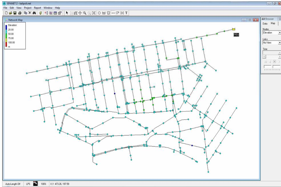
Figure 1. Hydraulic model of Kalipoli's DMA, using Epanet 2
