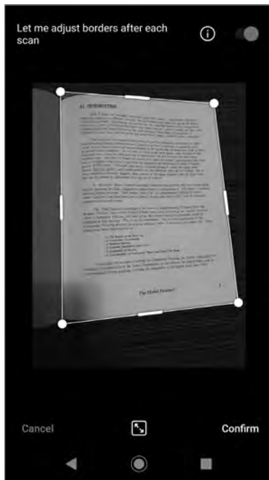
Figure 8: Many scanning apps include tools such as edge detection and de-skewing to improve image quality.
