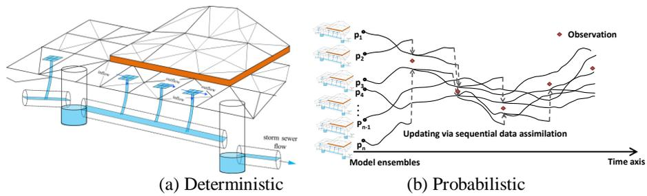
Figure 1. Concept of deterministic and probabilistic urban inundation modeling
