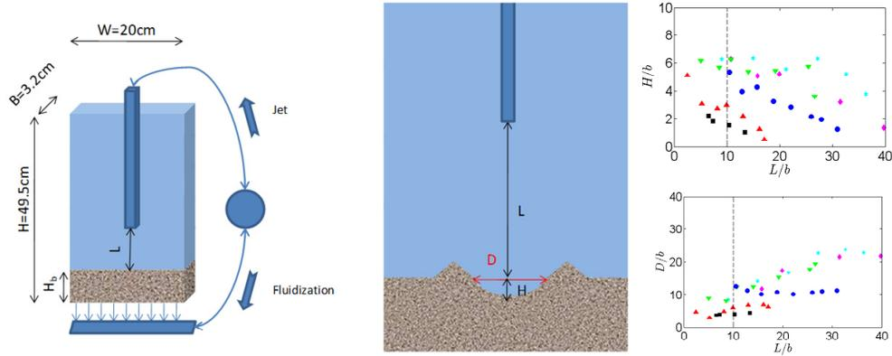
Figure 1. Experiment set up (left), definition of crater sizes (middle), results (right) in quasi-2D plane jet. Distance,  $L$ , depth,  $H$ , and width,  $D$  are divided by the jet nozzle size,  $b=4\text{mm}$ . The jet Reynolds number  $\text{Re}_j = 630$  (■),  $940$  (▲),  $1260$  (●),  $1570$  (▼),  $1730$  (◆), and  $1890$  (★) based on  $b$  and mean velocity  $U_j$ .
