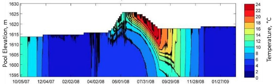
Figure 2. Example time series of reservoir pool temperature profile drawdown near the dam outlet for a moderately wet hydrologic year.
