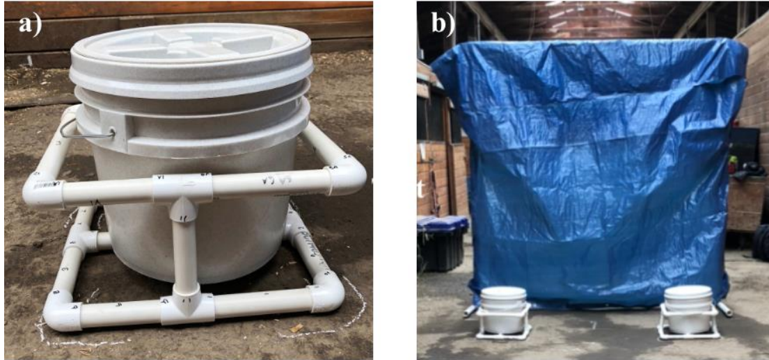
Figure 1. Photographs of experimental materials, including a) the PVC-pipe apparatus and bucket and b) the PVC-pipe partition and tarp.
