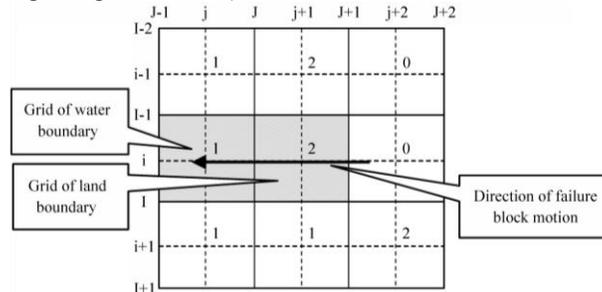
Figure 2 Classification of the bank failure grid
