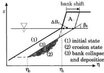
Figure 1 The model of bank failure by Hasegawa (1981)
