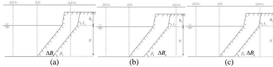
Figure 3 Calculation methods for bank erosion
