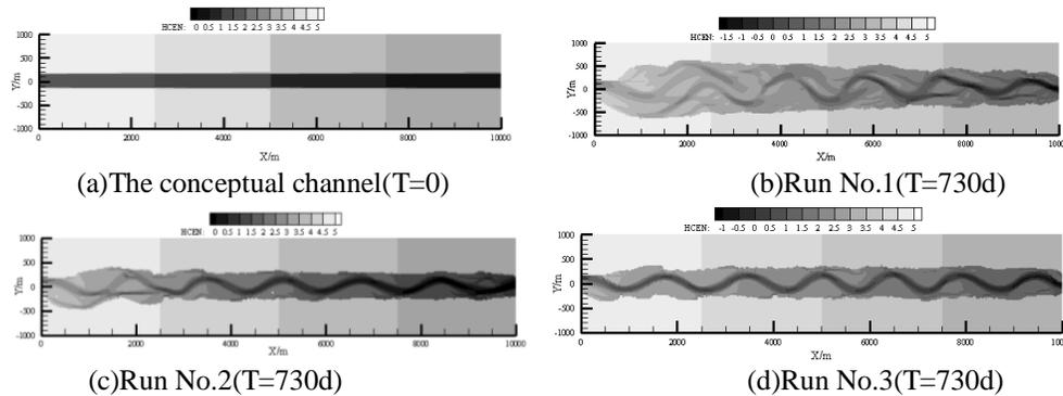
Figure 4 Simulated channel patterns after 730 days
