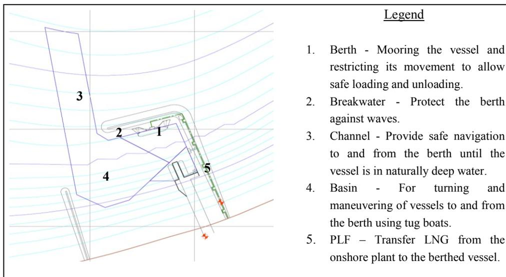
Figure 1. LNG terminal with berth 1150m offshore
