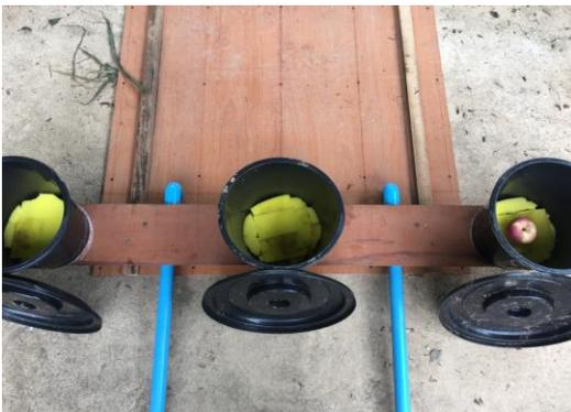
*Figure 4.* Photograph detailing apparatus with sponges lining the buckets. Lids are depicted in the vertical test position. An object (i.e. reward) is in bucket C.
