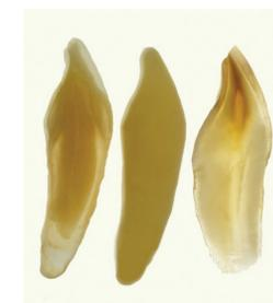
Figure 7. Natural Tooth Cross Section (Right). Feldspathic Cross Section (Center). Zirconia Cross Section (left)
