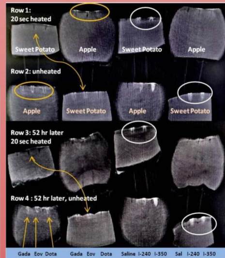
None of the Gd contrasts stay localized in both heated samples (yellow arrows) while Iodine contrast stay on heated sweet potato only (elliptical markers) but not on apples, contrast mechanisms are different, Iodine is chelating more metal ions in sweet potato.
