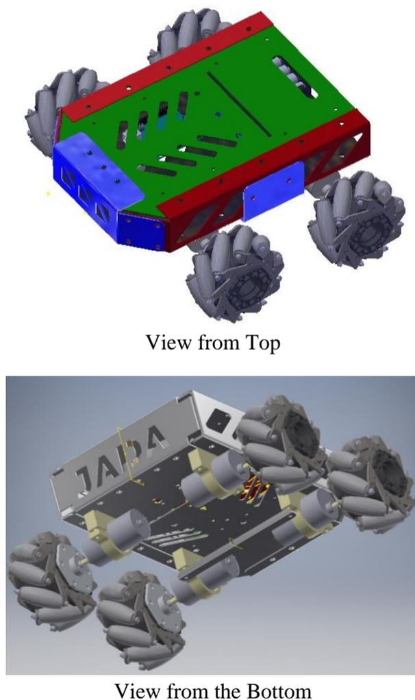
Figure 2 Computer-Aided Virtual Design Model of Robot Chassis using Sheet Metal
