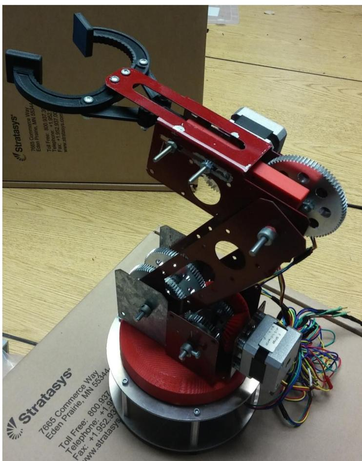
Figure 3 Custom-made Robotic Arm Using Stepper Motors
