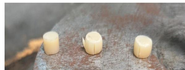
Figure 5. Horizontally printed specimens
