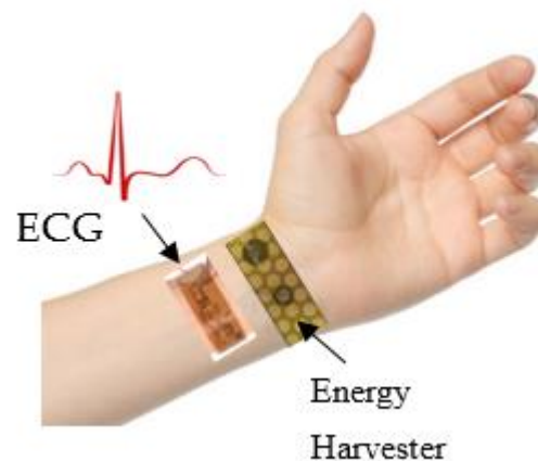
Figure 1. Illustration of a self-powered wearable electrocardiography (ECG) system. The ZnO energy harvester is intended to be placed on the skin of the arm.
