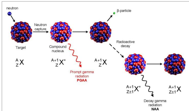
Figure 2. Neutron Activation of heavy metals from a research article shows distinctive gamma-radiation and the decay times of each specific radionuclide produced [Reference 4, Table 1].
