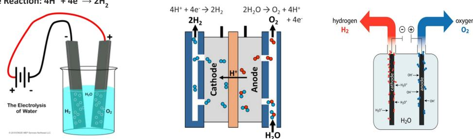
Figure 1. Left: Schematic representation of a simple water electrolysis. Center and right: Schematic representation of a fuel cell
