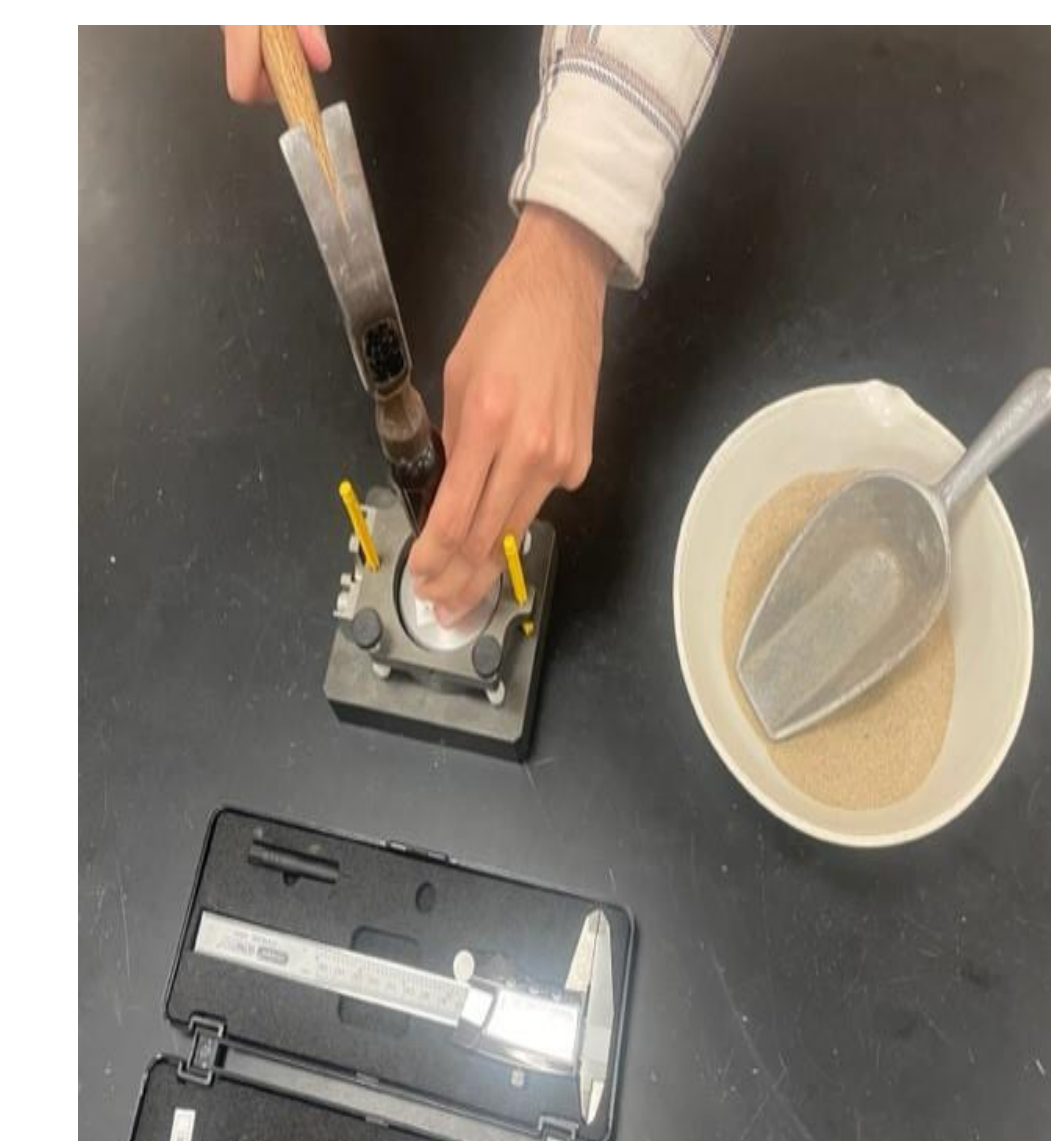
Fig 11: Compacting sample inside direct shear box
